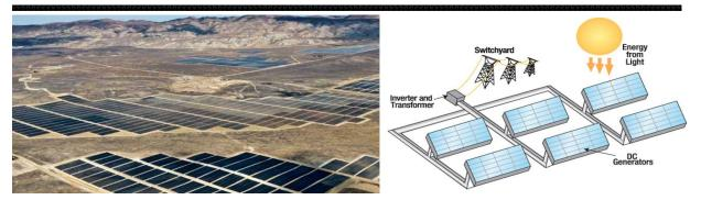
L ast issue we talked about thermal solar power plants utilizing mirrors to concentrate the suns power to a single point to produce power. Closer to home, all the solar power generating facilities in Eastern Kern County, currently, utilize photovoltaic (PV) cells. Covering acres of land, PV cells utilize specially treated sili-
